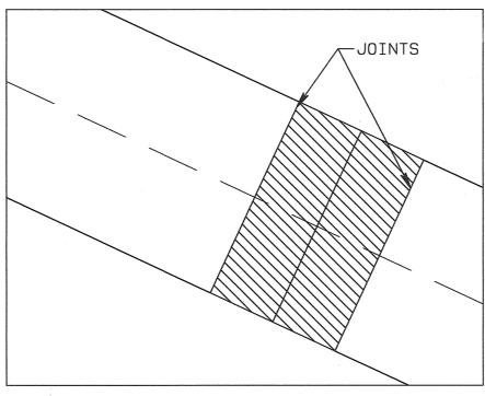
IN CONCRETE PAVEMENTS, REMOVE SECTIONS TO EXISTING JOINTS, OR NEW SAW CUT JOINTS AT MID-SLAB, THAT ARE IN GOOD REPAIR. IN DAMAGED CONCRETE, THE LIMITS OF REMOVAL SHOULD BE DETERMINED IN THE FIELD BY CITY INSPECTIONS.
