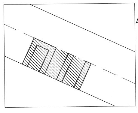
1. IN THE CASE OF A SERIES OF PATCHES OR PATCHES FOR SERVICE LINES OFF A MAIN TRENCH, REPAIR THE PAVEMENT OVER THE PATCHES BY GRINDING AND OVERLAY WHEN THE SPACING BETWEEN THE PATCHES IS LESS THAN 10 FEET. IN CASES WHERE THE EXISTING PAVEMENT IS IN POOR CONDITION (IN THE STRATEGIC PAVING PLAN) AND MAY REQUIRE OVERLAY WITHIN THE NEXT FEW YEARS, THIS REQUIREMENT MAY BE MODIFIED OR WAIVED BY THE CITY ENGINEER.
