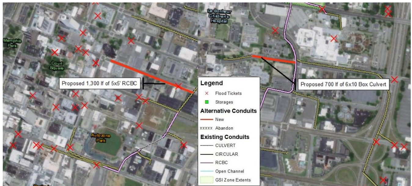
Figure 3-14 Scenario 6 – Areas with Potentially Surcharged Pipes (Left, W Jefferson Ave; Right, E Jefferson Ave)
